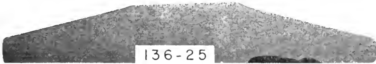
Fig. 4 (Investigation 136-25)—Photograph of a transverse section cut from the base of the rail adjacent to the fractured face. This section etched in a 10 percent nital solution, shows several electrode burns.
